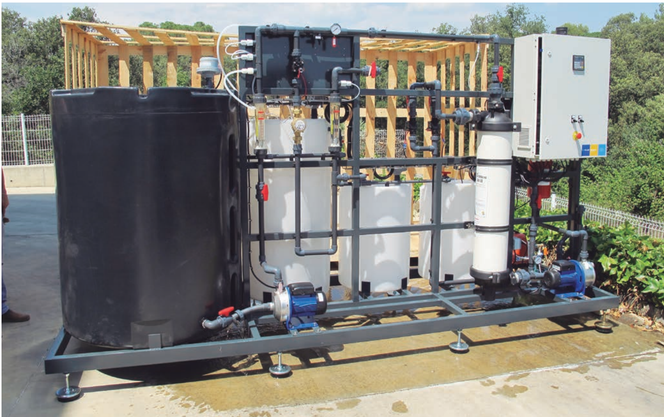
Ultrafiltration system of 4.000 l/day for the purification of drinking water installed in Uganda.
